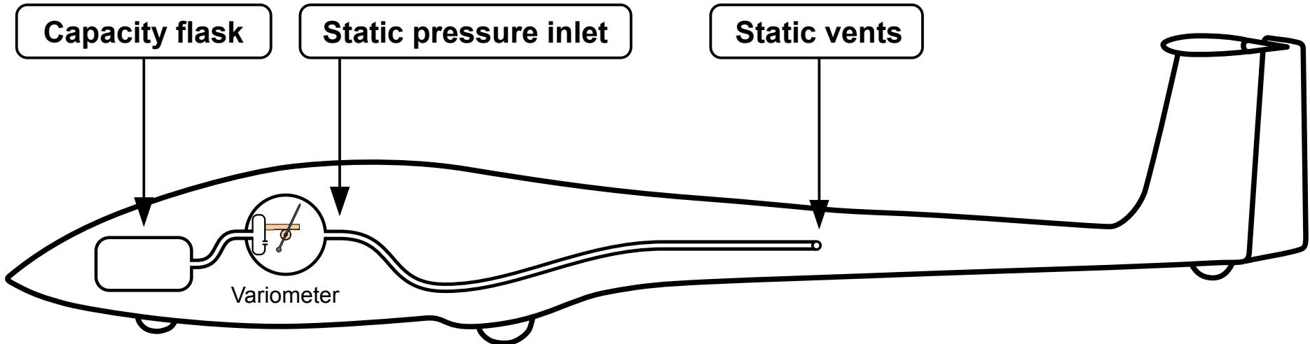
1 A variometer that is connected to the pipework shown above is termed as being **uncompensated**.
