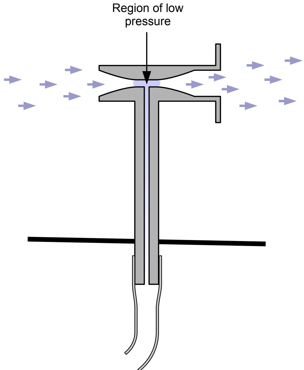
2 The faster the aircraft flies the lower the pressure over the vent hole(s) relative to the surrounding air.
