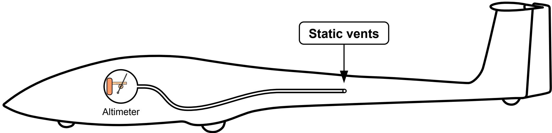
1 When designing a glider, the engineers will try to find a location on the fuselage where the passing airflow exerts a pressure on the aircraft's surface that is close to local atmospheric. They do this using a combination of their experience, calculations and test results. On a glider, such a point is often located about half way down the tail boom.
